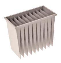
Green Flo bag filter made of PLA for low pressure drop. Filter class (F7) ePM1 50% on both supply and extract air. The filters are pressed against the sealing strip in the casing.
