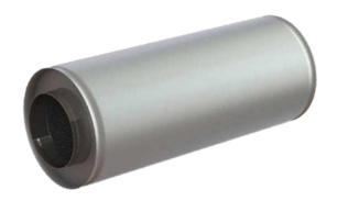
The silencer is a straight circular duct silencer with 50 mm mineral wool filling. Duct connections have rubber seals. The silencer consists of a perforated sheet metal pipe surrounded by a galvanized sheet steel mantle and end pieces sandwiching mineral wool covered with nonwoven fabric to prevent fiber migration. Fire resistance rating El30.
