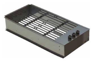
The electric heater has built-in control equipment for power control. The element is made of stainless steel. The heater has two thermal overload protection devices, one with an automatic reset and one with a manual reset.
